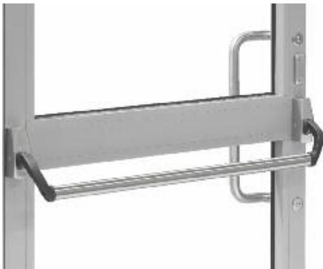
**Specification:** these doors should be fitted with a locking unit that is operable from the inside with a panic bar. The bar – NOT THE COMPLETE UNIT - should extend a minimum of 60% across the width of the door. Exit should be possible at a single push at anywhere on the bar. These doors must open outwards to conform with the standard.
